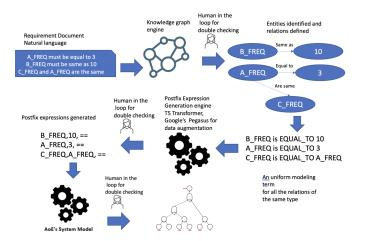
Figure 4: Machine Learning Example Pipeline.
